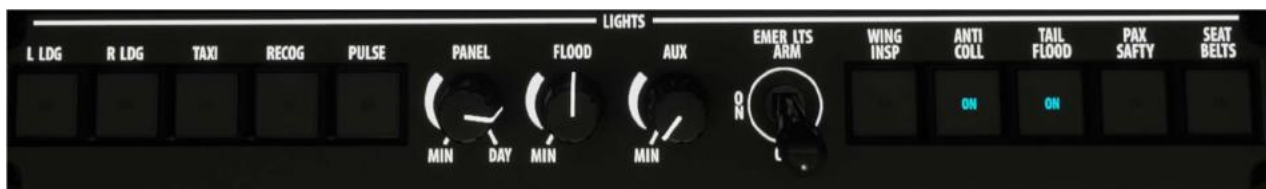
Fig 16-3-2 – Overhead lighting panel
