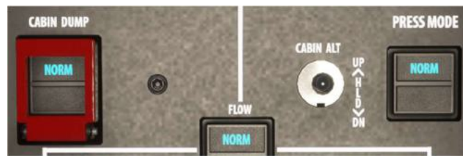
Fig 11-4-2 – Cabin Altitude pedestal controls
