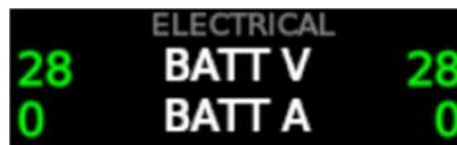
Fig 5-6-2 – Electrical EIS Display
