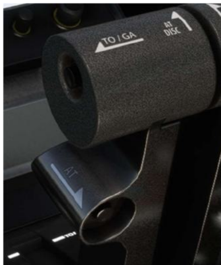
Fig 6-4-2 – Location of the TO/GA button (handle, left side) and AT arm button (handle arm, left side, facing aft)
